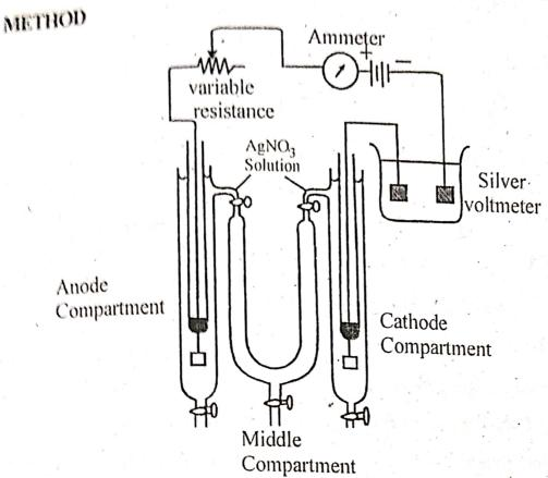
The Hittorf apparatus is shown in figure. It consists of two vertical glass tubes connected together through a U tube in the middle. The end tubes contain anode and cathode and consitute anodic and cathodic compartments. The U tube constitutes the middle compartment.
